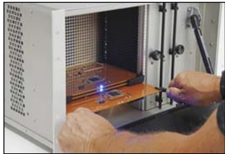
Installing an output expansion switch blade
